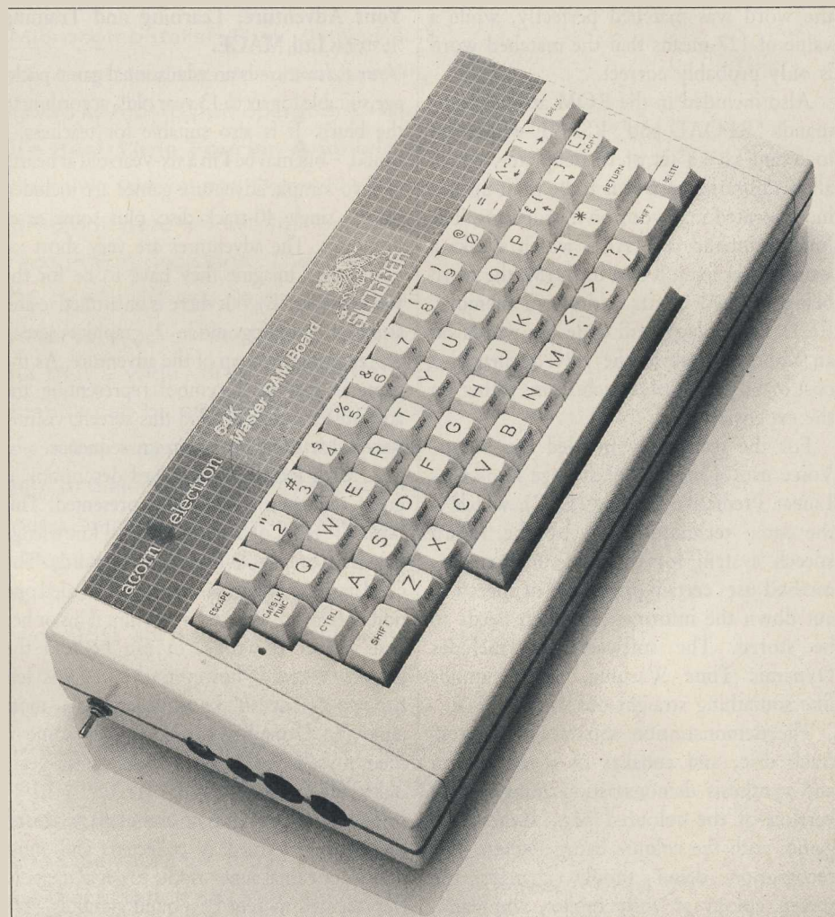
The only signs of the Slogger are the switch and stick-on label
