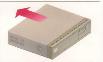
Some models of A5000 have a metal EMC case shield which fits over the inner case. To remove this, unscrew the five fixing screws on the righthand side of the computer, as seen from the rear. The shield has interleaved tabs which fit around the edges of the case. Slide the shield off the computer carefully; there is a hole on the top to help you slide the shield off by inserting a screwdriver.
