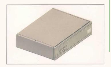
On **300-series (305, 310), 440s and 400/1-series Archimedes** computers, the top cover is held in place by three screws at the top rear, and one screw on either side of the cover, towards the front. These must be removed before the cover can be slid off. (On some early Archimedes you will need to adjust the position of the backplate on the card to ensure that when the card is installed and bolted in place, the connector is seated correctly and the backplane vertical.)
