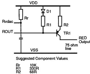
Figure 7: suggested video output circuit for VIDC2.
