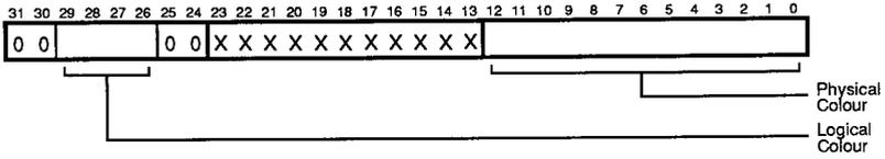
In 1,2 & 4 bits per pixel mode, data bits **D[0:12]** define the physical colour corresponding to that logical colour.
