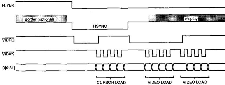
Figure 3: Cursor DMA at the Start of a Frame
