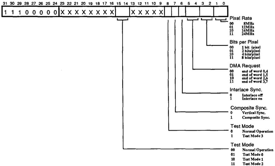
This register defines the basic operating mode controls. A total of 11 bits are defined, and three of these are for test purposes only. Note that bit 8 in the SFR must also be set before the device can operate correctly.
