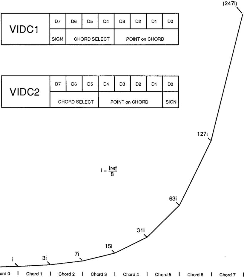
The outputs are current sinks. The magnitude of the output is a function of the sound reference input current. The reference current is equal to the step size in the highest chord, which is 8i in the figure above.
