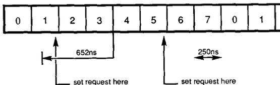
Figure 4: FIFO operating at 16MBytes  $s^{-1}$ .
