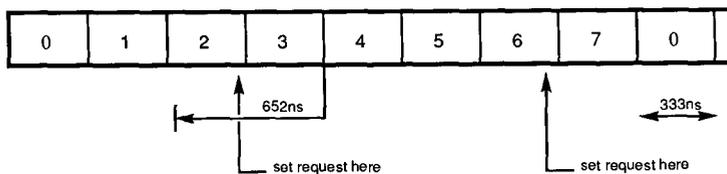
Figure 5: FIFO operating at 12MBytes  $s^{-1}$ .
