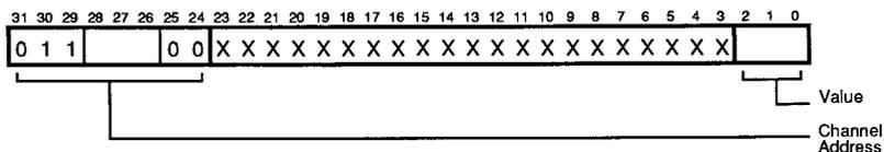
These 8 registers define the stereo image position for each of the 8 possible channels as shown in Table 2.
