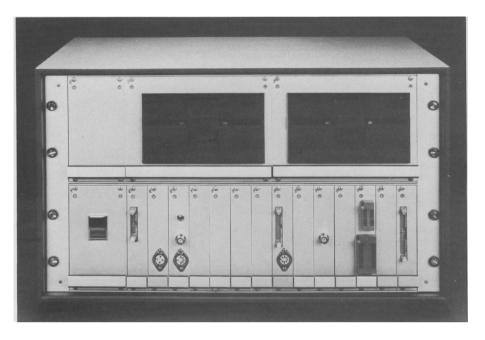
The System 4 is housed in a double height rack with facilities for up to 14 Eurocards. The basic system has as standard two floppy disk drives, power supplies, card frame buffered backplane, 6502 CPU, VDU interface, 16K RAM and disk controller. A DOS controls both disk drives, and a disk with utilities programs including disk copy is supplied with each system.
