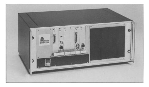
The System 5 is housed in a 4U, 19" card frame with seven Eurocard slots. There is provision for one or two mini-floppy disk drives allowing systems with from 100 to 800K bytes of disk memory to be supplied depending upon the type of drive used. Also used in the system is a switch mode power supply Eurocard giving 5 and 12v supplies, larger systems with two disks drives will have two of these supplied.
