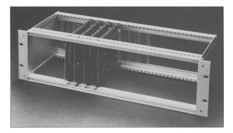
The System 2 has many applications in the area where audio cassette based storage is required. It also provides a basis for the addition of more Eurocards.
