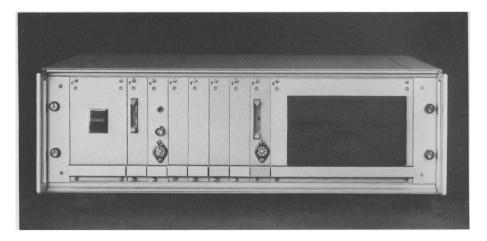
The System 3 in its basic form is a system driving a single disk. The hardware consists of a card frame, backplane with 4 sockets, 6502 CPU, VDU interface, 8K RAM, floppy disk module, DOS and resident 4K BASIC.
