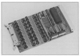
in the range 6 to 48v. A catching diode on each output allows inductive loads to be used. In input mode each connection is driven by contact closures to the remote supply common. An LED indicates the state of each connection in input or output mode.
