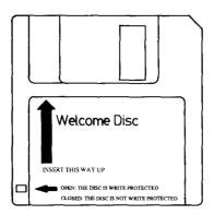
The drawing above shows you the correct way to insert a floppy disc into the drive. The disc enters the drive in the direction the arrow is pointing. Follow these steps:
