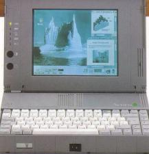
It comes with a sturdy, easily replaced, rechargeable battery pack which under normal use will provide 2.5 - 3.5 hours of uninterrupted use with additional battery packs being available to accommodate longer periods away from a mains supply.
