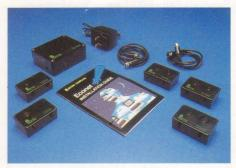
Filestore provides advanced and extensive File server and printer server facilities to Econet system users. Filestore E01S can act as the core unit of a network or plug straight into an existing network to provide extra capacity. Mass data storage on hard disc is provided by connecting Filestore E40S or E60S units with 40–60 Mb respectively which can be added as demand for storage capacity grows.
