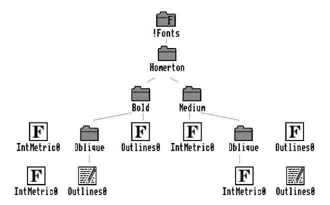
Although the structure looks confusing all that is required is to work down the structure one directory at a time adding the lines to the structure information. There are four typefaces in the Homerton font which is quite normal for the standard, commonly used fonts. The four lines of the Homerton font structure would be as follows:
