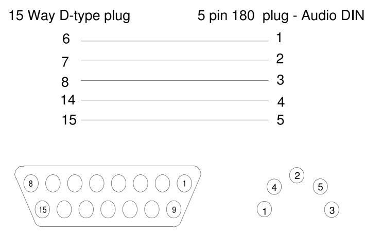
NOTE: Connections as viewed from back of connector (solder side).
